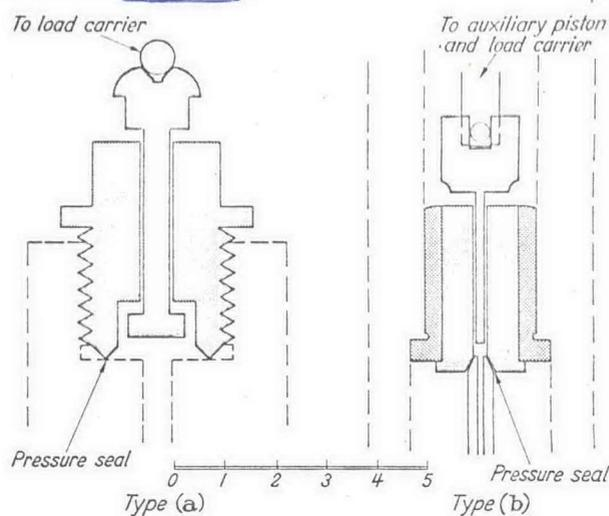
Fig. 2. Diagrams of piston-cylinder assemblies (Scale of cm)
